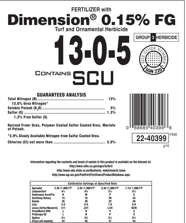
These settings were calibrated and field tested. However, age and condition of spreader, speed of operation and evenness of terrain may require slightly different settings for desired coverage.
